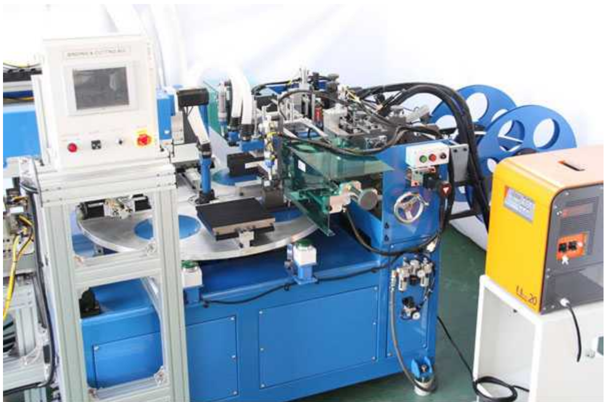
MAIN INDEX WITH PLEATED PAPER CORE JIG & PAPER RIBON UNCOILER
