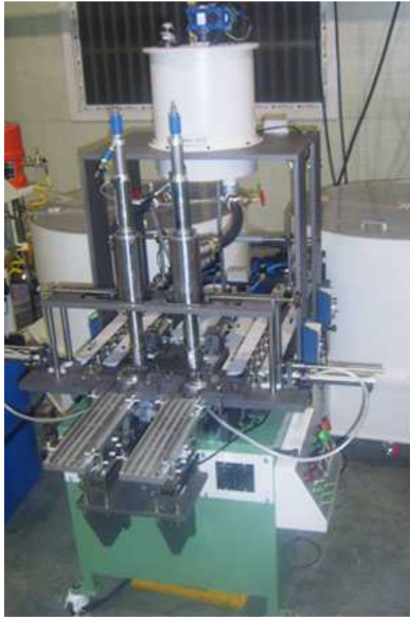
Main PVC Sol Dispenser M/C Photo with Auto Loading Parts Feeding Device
